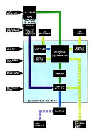
In its automatic mode the XG-7 is an aperture-priority camera. This simply means that you set the lens opening while the XG-7 sets the shutter speed.
