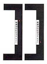
The upper LED triangle lights to warn against overexposure, and the shutter will lock until you properly adjust the aperture. The lower LED triangle warns against underexposure.
