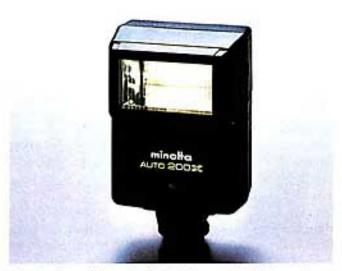
Slip the Auto Electrollash 200X onto the XG-7 and turn it on. In manual, the Hi setting (Guide Number 33 in feet at ASA 25) is for conventional flash shooting. The Lo setting (Guide Number 12 in feet at ASA 25) is for winder synch and will recycle as fast as two frames per second.
